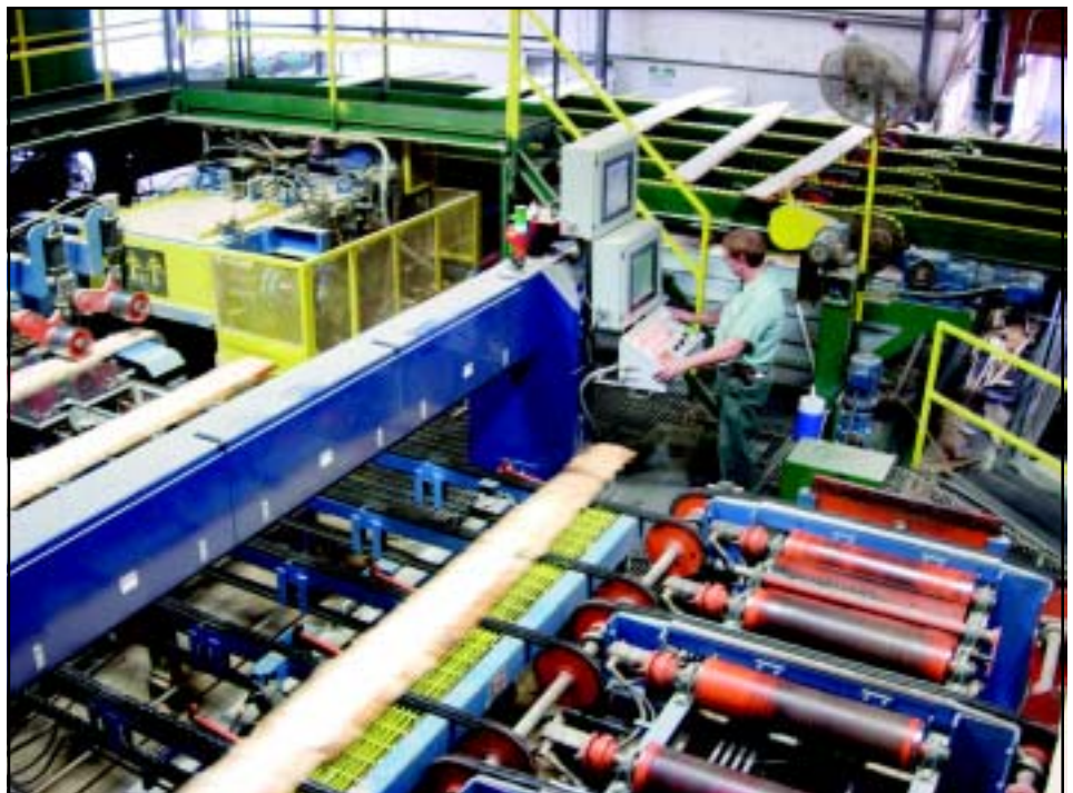
Flitches move from right to left under INOVEC edger optimizer prior to entering the Timber Machine Technologies (TMT) three-saw edger, visible in top left of photo.
