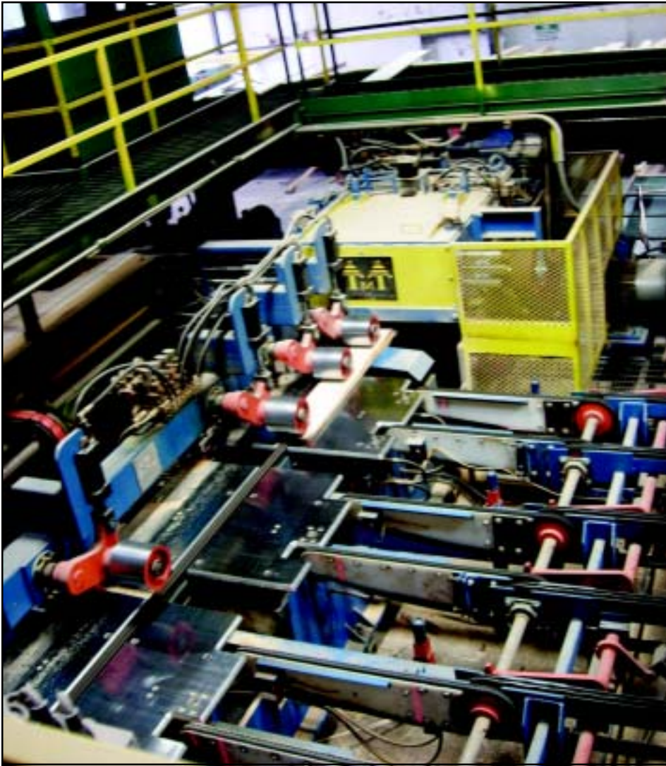
View of the in-feed of the TMT edger. The edging process is controlled with the INOVEC WaneMaster G3 optimization system.
