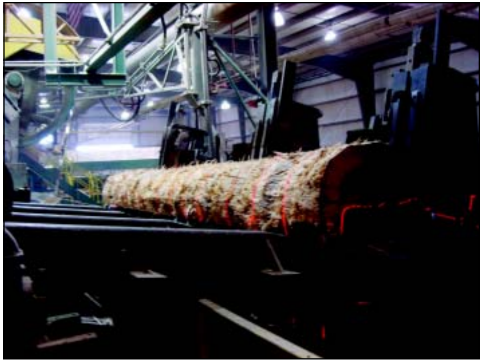
Scanner projects laser lines onto a log on the carriage; the head rig is optimized with the INOVEC YieldMaster system with StereoScan 3-D log scanning technology.
